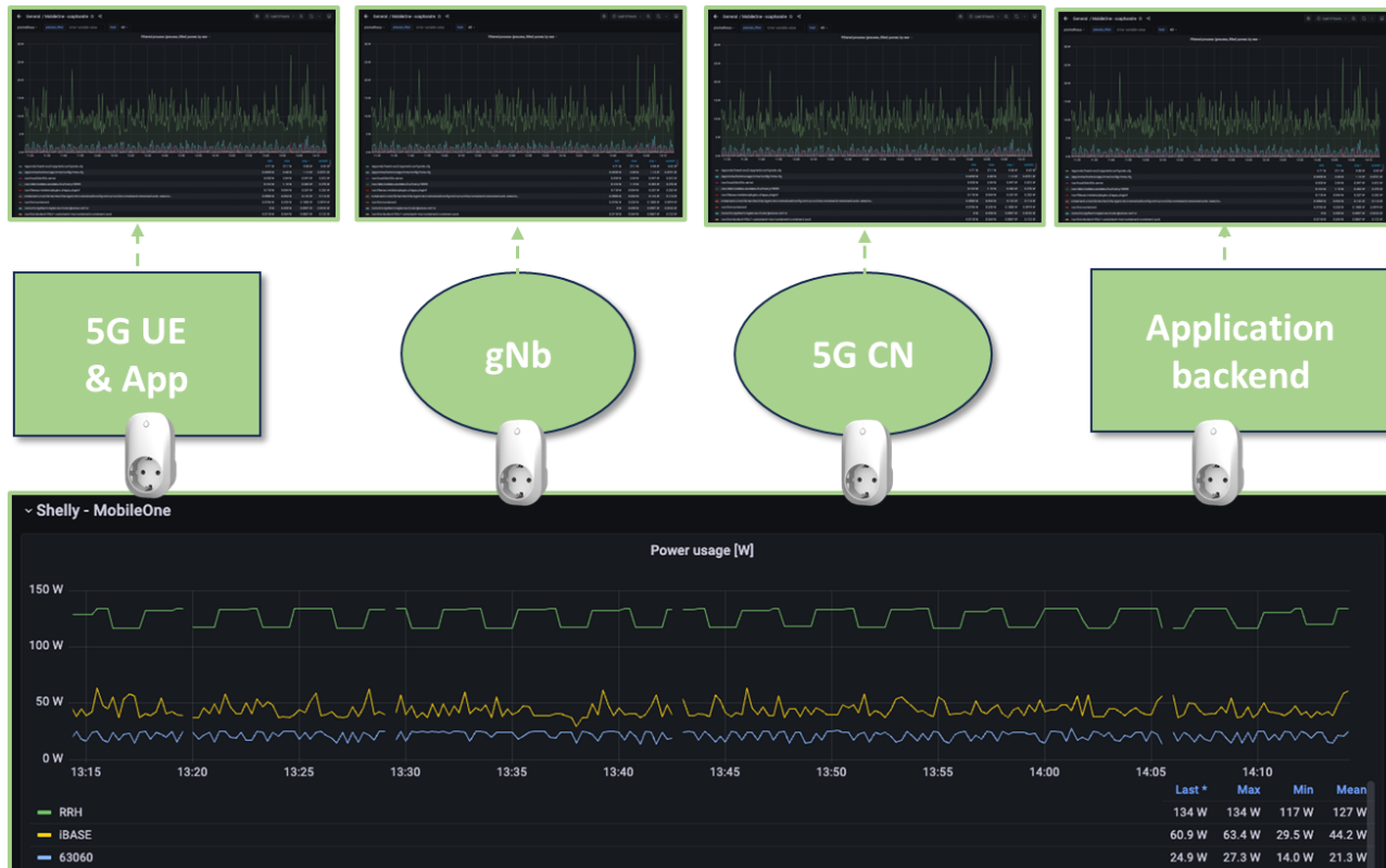
Figure 5-29: Measuring power consumption taking into consideration end-to-end perspective.
